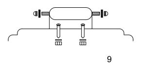
Loosely fit the right Q and Left hand wind shield C via the lower fixing holes using 2 off M6 x 10mm screws 99, washer-nuts dd for the rear holes, 2 off M6 x 16mm screws, washer-nuts for the side locating holes.
